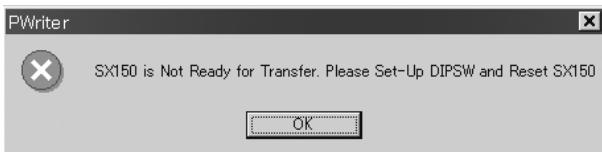
This error message is displayed when the matrix switcher's mode is not “SX150 SOFTWARE UPLOAD”.
