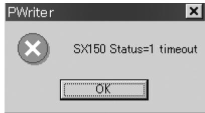
This error message is displayed when a specified time has passed since you started installing SX150A Program Writer/updating the firmware. The following are the timeout error statuses.
